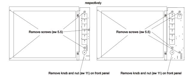
Fig. 3 (Removing a TFT display incl. touch screen)
