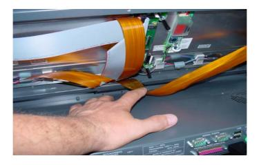
● You have to re-locate the 3 threaded pins for the main board - 3 bores on the DFI main board are on different locations compared to the ASUS board.
