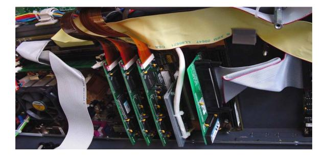
● As the 3 display ribbon cables cannot be crossed over, it would be best to pull out the cables from the guiding shaft (from the rear side of th econsole after removing the cover plate) and insert them in reverse order, to facilitate connecting the cables to the display adapters.
