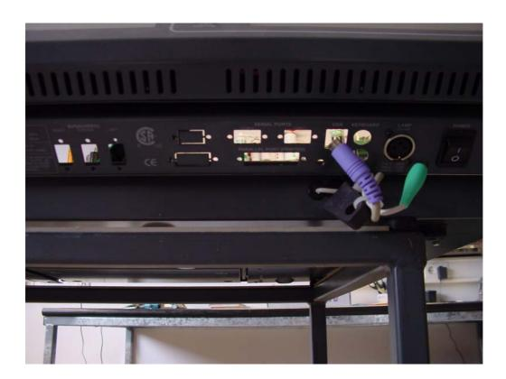
■ Insert 2 cable ties (for the mouse and keyboard cables) through the two bore holes of the spacer block and tighten the two cables.
